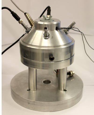
(a) Structure and sensors.
