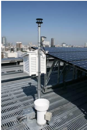
Figure 7 Picture of roof-top weather station used to measure ambient conditions used in the control system.
