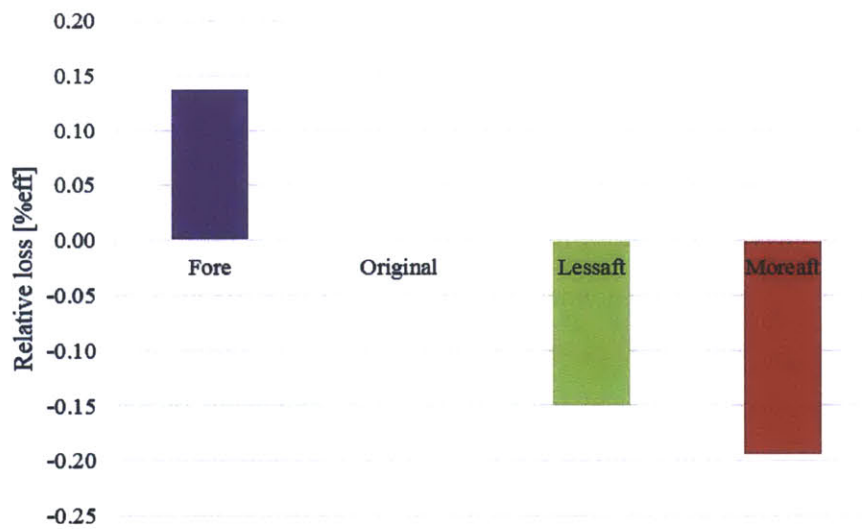
Figure 3-9: Relative loss benefit of tip leakage flow formation delay
