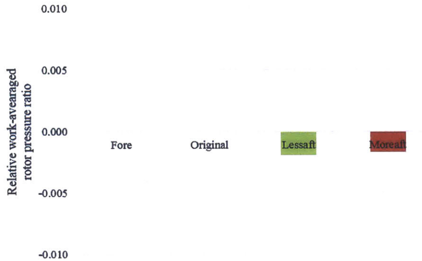
Figure 3-4: Negligible changes in relative work-averaged rotor pressure ratio in the four rotor blade designs
