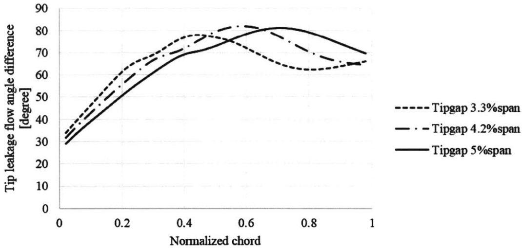
Figure 3-18: Similarity of chordwise distribution of tip leakage flow angle mismatch at three tip clearance sizes
