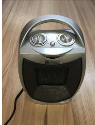
(a) Space Heater used as Internal Load
