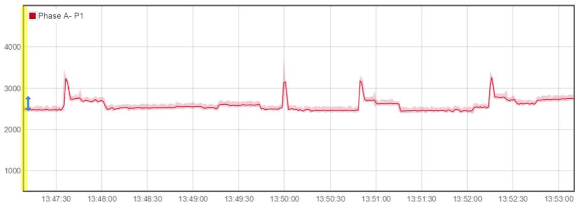
Figure 5-5: MCM Number 2 AC Transients
