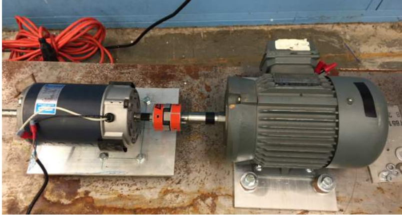
Figure 3-8: Original MMTP with Multiple Subbases
