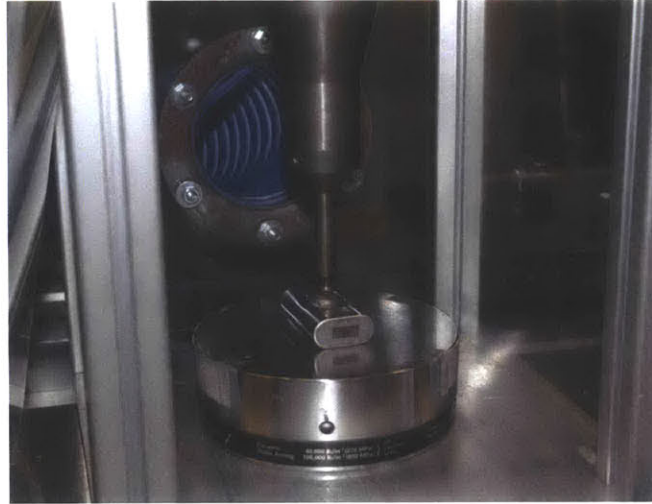
Figure 3-3: Elliptic Cell Punch Indentation Test Setup
