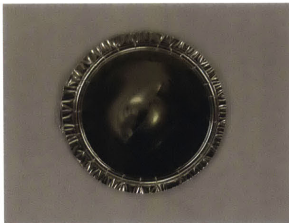
Figure 3-40: Elliptic Aluminum Biaxial Test Sample 5
