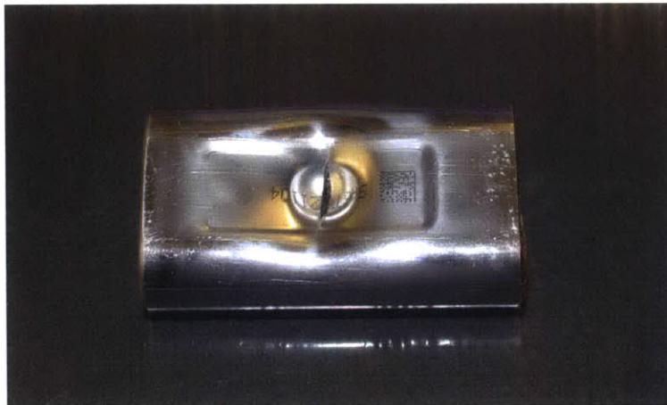
Figure 3-9: Elliptic Cell Damage from Punch Test
