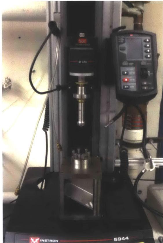
Figure 1-4: Instron Test Machine with Biaxial Punch
