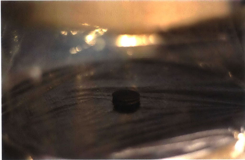
Figure 3-48: Elliptic Coated Metal Compression Test Samples
