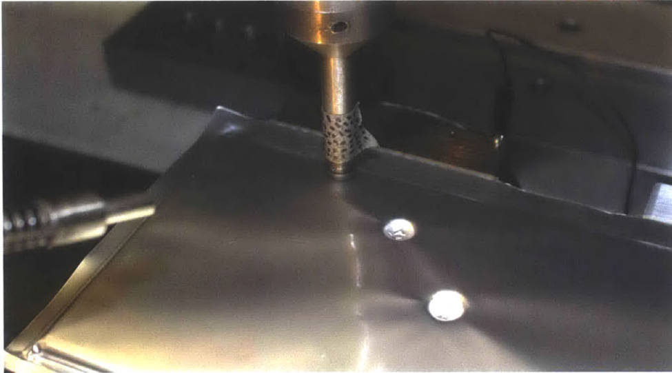
Figure 4-5: Pouch Dry Cell Hemispherical Punch Test 3
