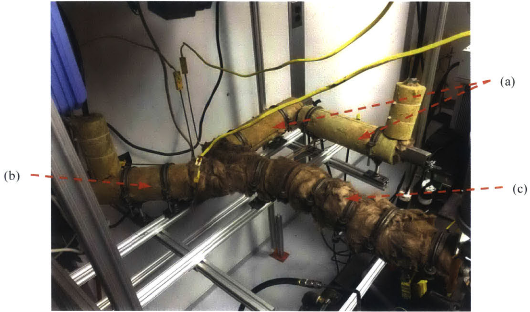
Figure 2-16. Gas process heaters and mineral wool insulation for spark-ignited engine cylinder. (a) air heater; (b) \text{CH}_4 + \text{H}_2 + \text{C}_2\text{H}_6 heater; (c) heat cable for mixed gas.
