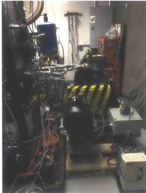
Figure 2-2. The Lister-Petter TR1 single-cylinder diesel engine was fixed to a separate pallet to the right of the cast iron T-slotted test bed. The intake composition and temperature control system is to the left of the engine. The data acquisition hardware and power supplies are on an instrument tower also to the left of the engine.
