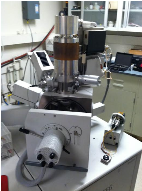
Figure 12.5. Environmental Scanning Electron Microscope (ESEM) at MIT used for imaging membrane fouling
