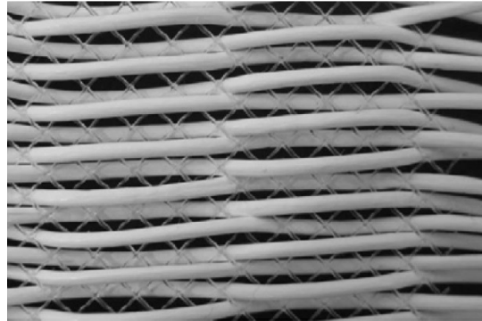
Figure 6.14. Example of mesh spacers used in hollow fiber MD experiments [37].
