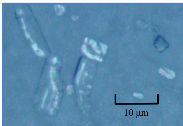
Figure 10.5. Microscope image of MD membrane after seawater experiments
