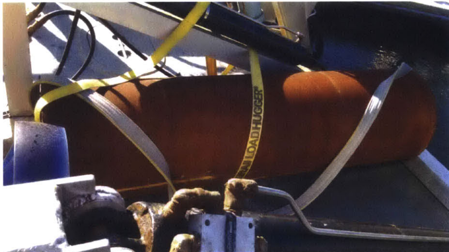
Figure 4-15: Open-ended steel pipe used as a target during the Massachusetts Bay experiment, sitting on the deck of the R/V Resolution . The pipe is 1.5 feet in diameter and 5 feet long.
