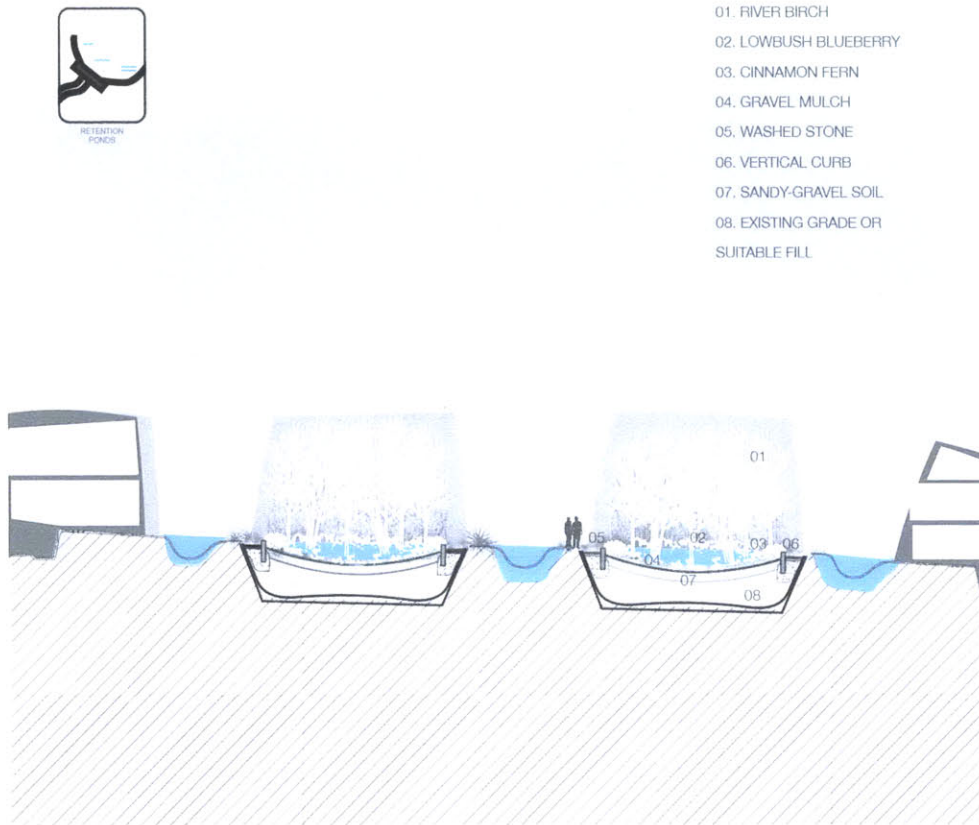
DETAIL SECTION THROUGH RESIDENTIAL BLOCK : INFILTRATION ISLANDS
