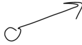
Figure 2-4: Components need not contain a whole number of strokes. Here, a vertex, edge, and arrow are drawn with a single stroke.
