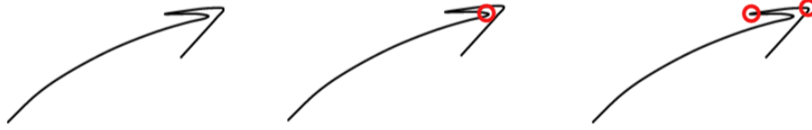
Figure 3-1: The arrow and edge on the left are drawn with a single stroke. There is one true segmentation point that occurs at the transition between these two components, as indicated by the circle in the middle image. The stroke has two other points, which are circled in the right image, that appear to have properties similar to those of the true segmentation point.
