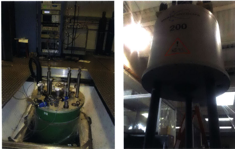
Figure 2-1: The cold-bore solenoidal magnet is shown on the left and the current warm-bore NMR magnet is shown on the right [5].
