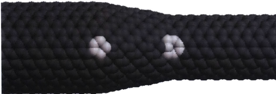
Figure 5-7: Nanoscale nozzle geometry proposed by Hanasaki and Nakatani, consisting of two CNTs joined at a convergent neck. Figure from [10].
