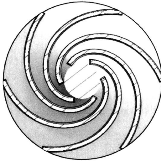
Figure 3-10: Bird's Eye Sectional View of Impeller, Showing Layout of the Vanes
