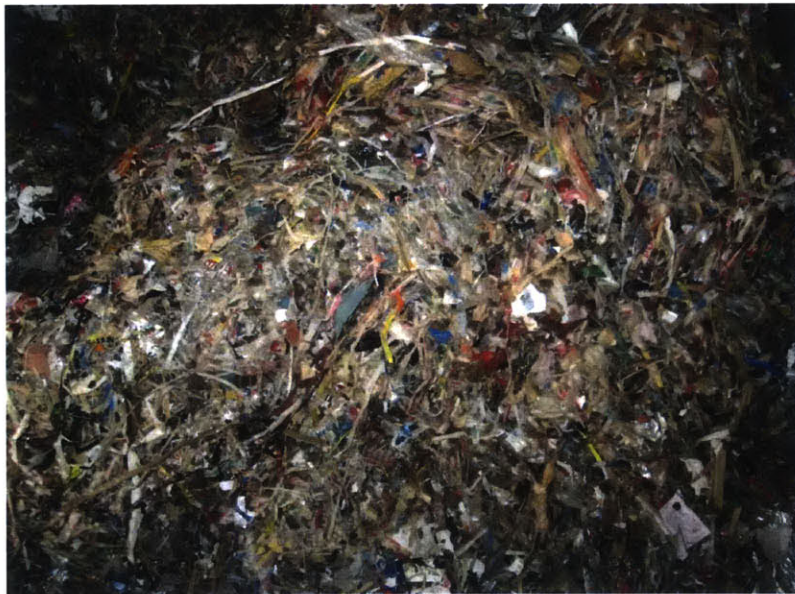
Figure 5 Waste plastic separated from the pulping process in a pulp & paper mill
