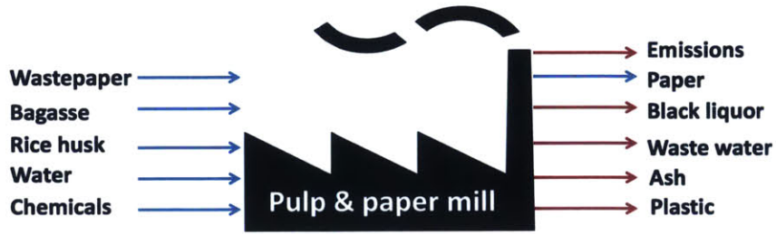
Figure 2 Material inflow and outflow from an SME pulp & paper mill
