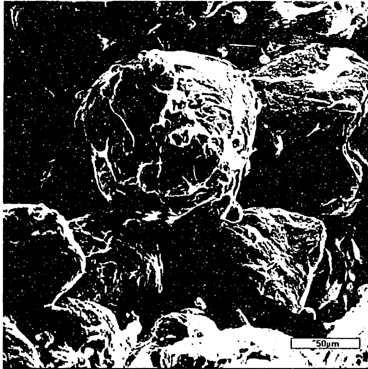
Figure 8.6: High magnification view of polymer surface between pillars
