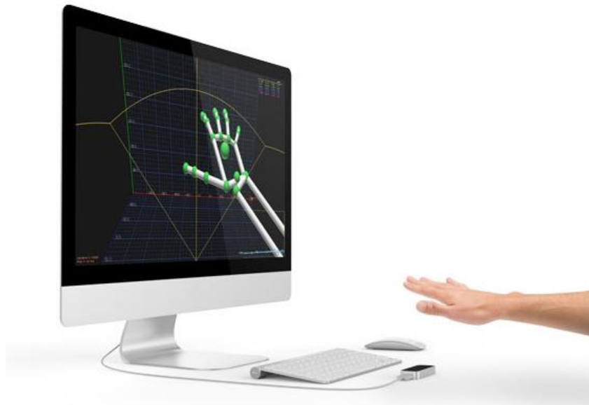
Figure 3: A Leap Motion and its visualization. https://www.leapmotion.com/
