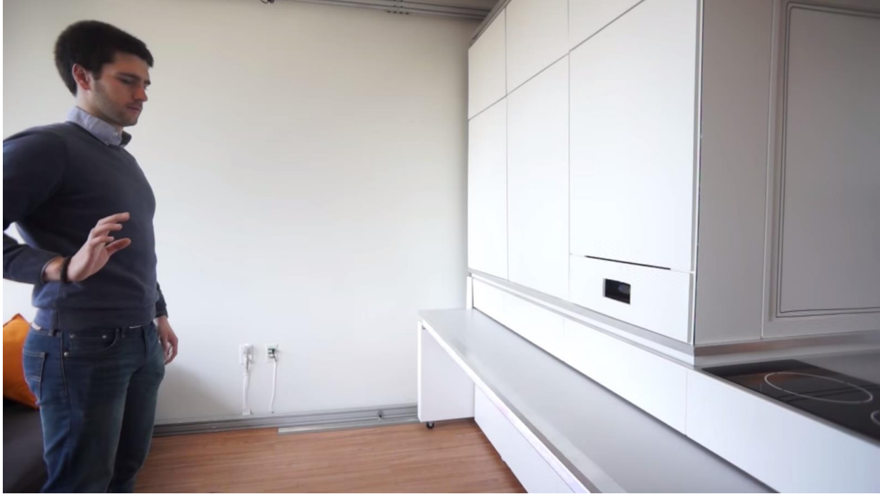
Figure 5: Table moving out in the CityHome 1 prototype because of pull gesture.
