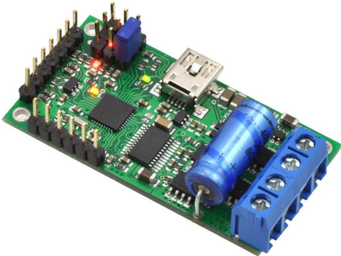
Figure 11: A simple motor controller from Pololu. https://www.pololu.com/product/1378
