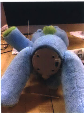
Figure 3-14. Acrylic base stabilizer screwed at the bottom of the robot with access to the power button
