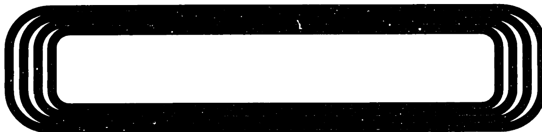
Figure 4-1: A schematic of the final coil design is shown. Cooling fluid flows into the page through the separated end-turns.
