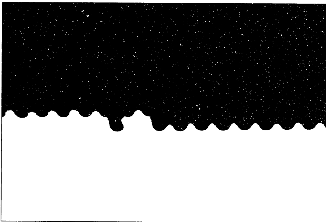
Figure 3.2: Image of Winding with Gap Error
