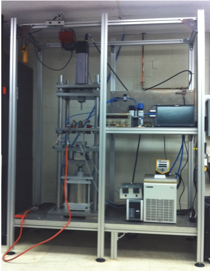
Figure B.1: Illustration of the injection-molding machine for preparation of injection-molded samples
