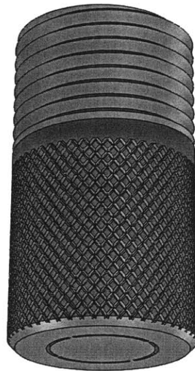
Figure A-3: Integrated spinneret head detail
