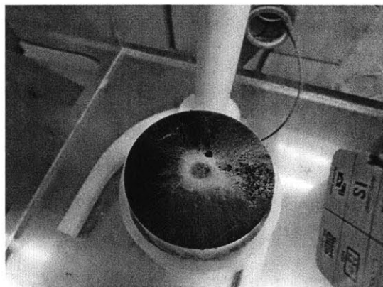
Figure 3-6: Fiber deposition around die orifice at edge
