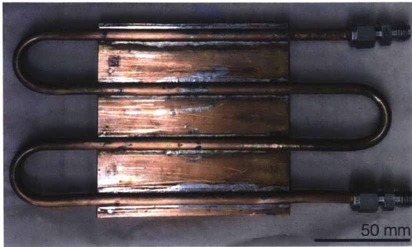
Figure 2. Cold stage used to remove waste heat from thermoelectric devices. The copper block used here is 100 mm x 100 mm x 9.5 mm. The copper tubing is one-quarter inch tubing. To ensure good thermal contact between the block and tubing, a one-quarter inch ball end mill was used to mill four semicircular channels in the block. The tubing was then bent to specifications and soldered into the block.
