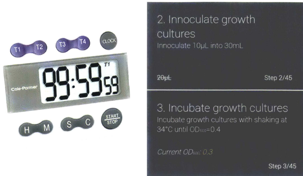
Figure 2-10: Left: A common lab timer. It consists of an LCD screen for displaying time, a buzzer and a few buttons to navigate through a couple of timers and start/stop them at will. Right: Sample notification integration where the user is informed of the timer's completion via SMS or through a heads-up display on Google Glass.
