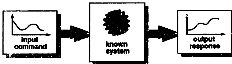
Figure 1.1: The feedforward control problem.
