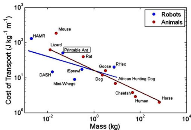
Fig. 8. COT versus mass for various legged robots and animals. Animal data adapted from [38], robot data from [39].
