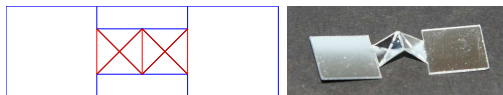
Fig. 6. This flexural element permits longitudinal compression as well as in-plane and out-of-plane rotations.
