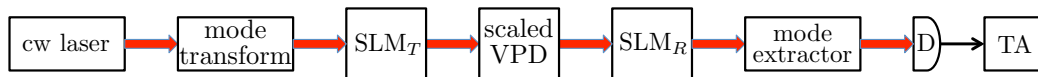
Figure 2: Notional setup for physical simulation of average intermodal cross talk. SLM_T and SLM_R : transmitter-pupil and receiver-pupil spatial light modulators. Scaled VPD: scaled vacuum-propagation diffraction. D: detector. TA: time average.
