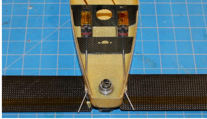
Figure 23: Rear wing assembled with control and deployment system
