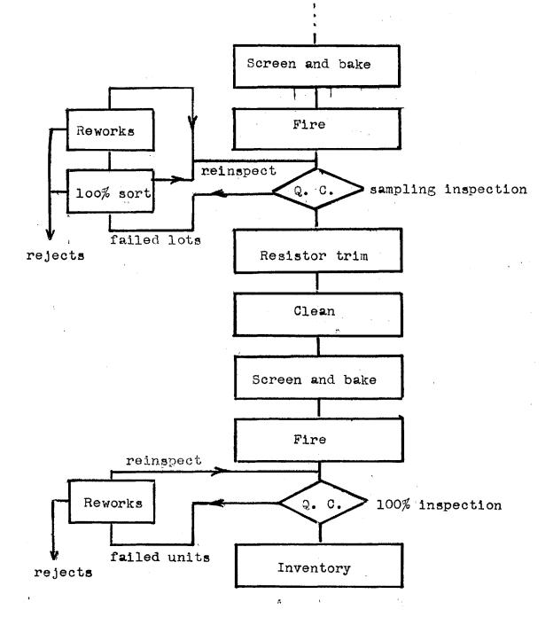
and then move to the next station to have a special capacitor attached. In this manner a unit moves thru the cycle gradually accumulating its active components. At the completion of the cycle a protective plastic is put over the circuit and it is moved to the finished goods inventory.
