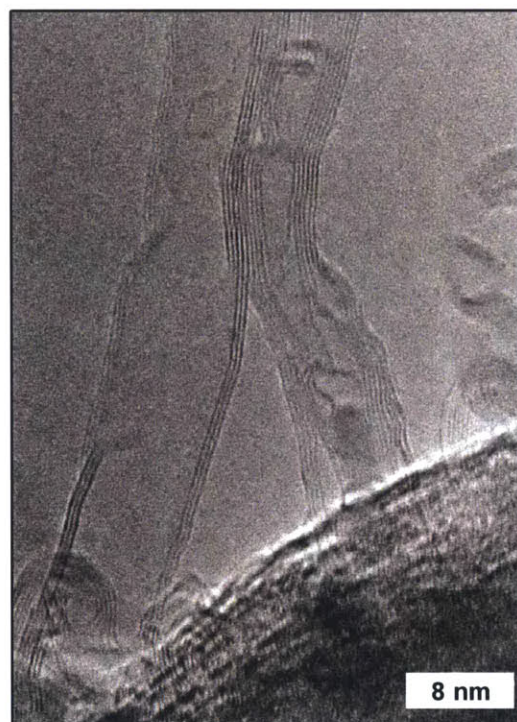
Figure 2.5 TEM image of two coupled CNTs, with the CNT on the right in compression as evidenced by buckles in its walls [courtesy of M. Bedewy]
