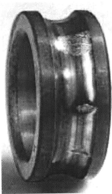
(a) Spalling due to abrasion
