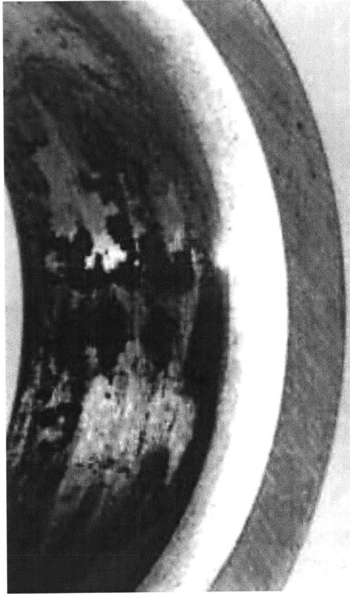
Figure 4-7: Extensive fretting corrosion in the bore of a self-aligning ball bearing [28].
