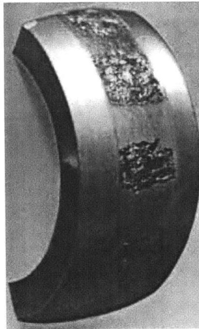
(b) Spalling due to galling
