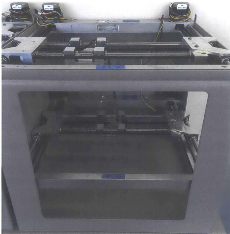
Figure 6-3: XY gantries double stacked within encasement.
