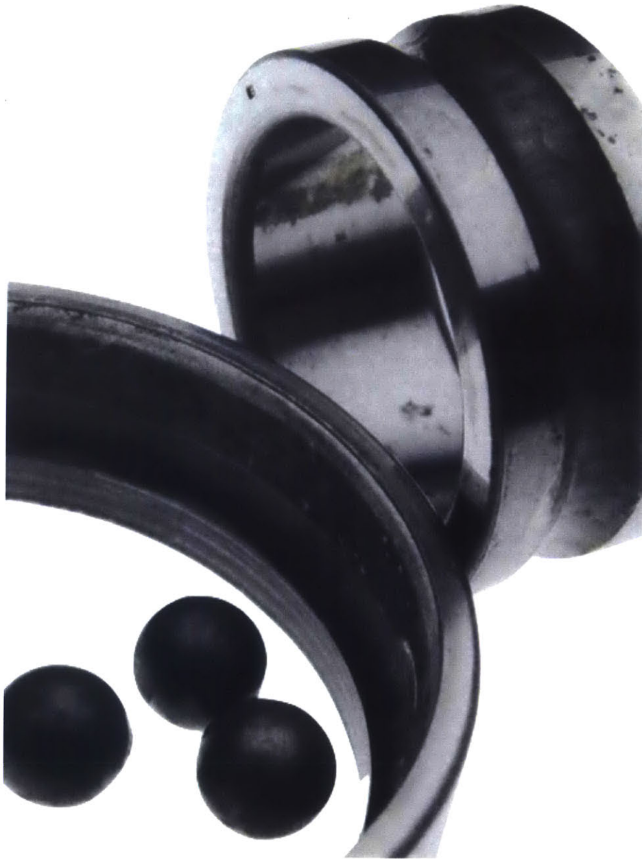
Figure 4-6: Corrosion on roller bearing raceways and balls as a result of moisture, as indicated by reddish-brown stains, flaking, and pitting [29].
