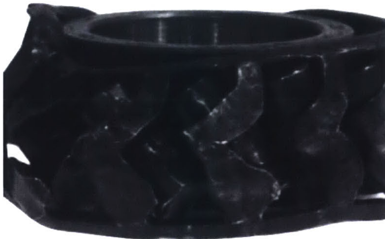
Figure 4-4: Complete bearing seizure due to continuous lubricant-free operation. Excessive heat from galling caused plastic flow and bearing cage deformation [30].
