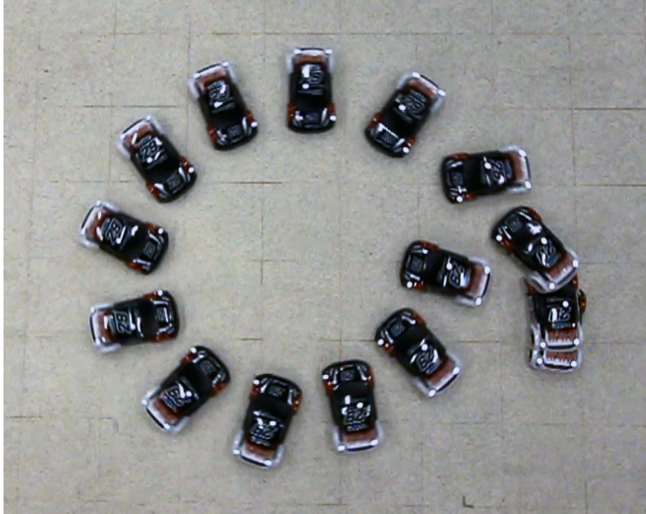
Figure 5-14: Results of Algorithm 6 applied to the real drifting car. Snapshots of the car every 0.25 seconds are shown. The vehicle starts from rest and quickly enters a controlled drifting motion with a 0.8 m radius.
