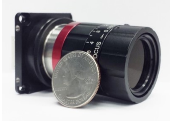
Figure 2-8: CubeSat-sized laser beacon camera utilized in NODE for ground tracking
