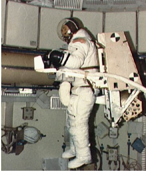
Figure 1-4: The Astronaut Maneuvering Research Vehicle (AMRV). The AMRV was flown inside the volume of the Skylab orbiting facility as part of the M509 Experiment on the Skylab 3 Mission, 1973 [5]. The AMRV featured 6 CMGs in three scissor-pair configurations for attitude control testing. Image courtesy of NASA.
