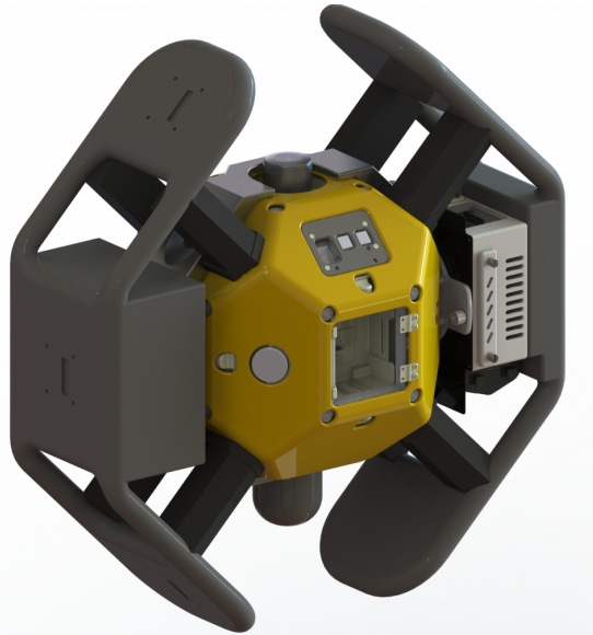
Figure 1-7: SPHERES and the Halo Expansion. Up to six peripherals can be interfaced with Halo and communicate with the central SPHERES satellite.
