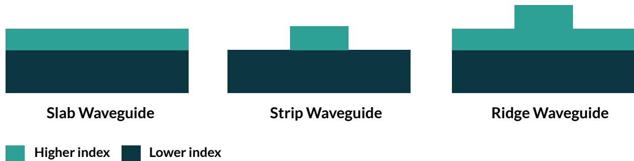
Figure 3.1: Schematic showing the three main types of waveguides. The waveguide core is comprised of a higher index material than the undercladding to confine the mode spatially. The work presented in this thesis uses strip (or channel) waveguides.
