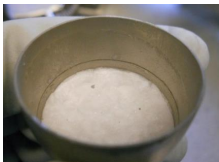
Figure 43 - 80/20 NaOH/NaI salt in a Ni-201 crucible after melting and before pulverization
