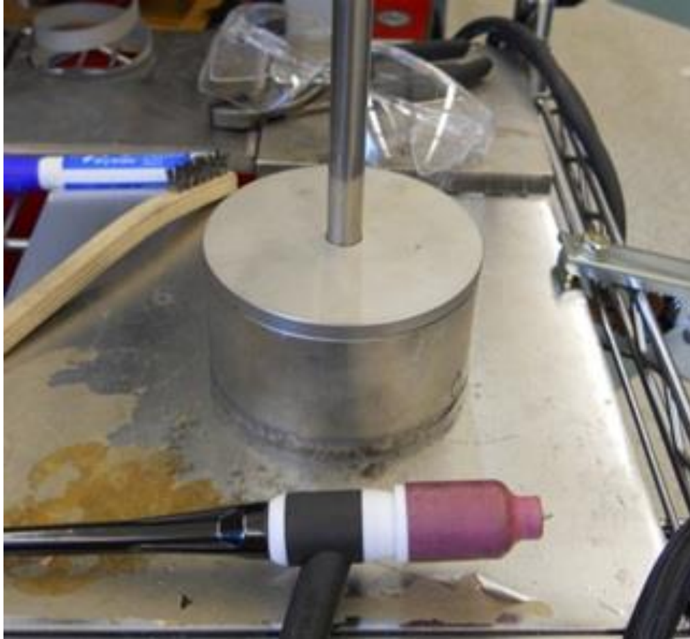
Figure 8 - Open air assembly of a 40 Ah liquid metal battery
