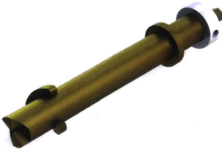
Figure 3-4: The right end of the key bit features a hexagonal shaft that functions as a generic point to which a torque-transmitting end effector may attach, and the gold and white rings keep the key bit attached to the vehicle. Finally, both geometric features protruding from either the side or the end of the key bit shaft at the left end of the key bit transmit torque and thrust to either the drilling piece or the tapping piece.
