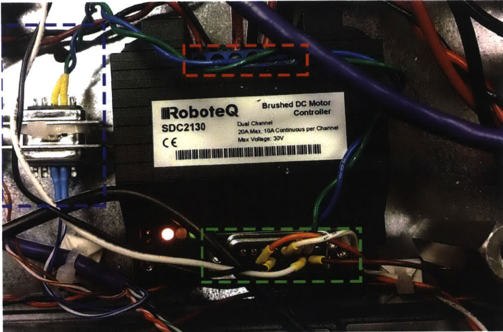
Figure 4-10: The RoboteQ SDC2130 Motor Controller acts as a hub through which motor commands are sent to either the linear actuator or the thrusters (red box), or analog string potentiometer data is received (green box). Communication is made with the Linux machine via USB connection (blue box).
