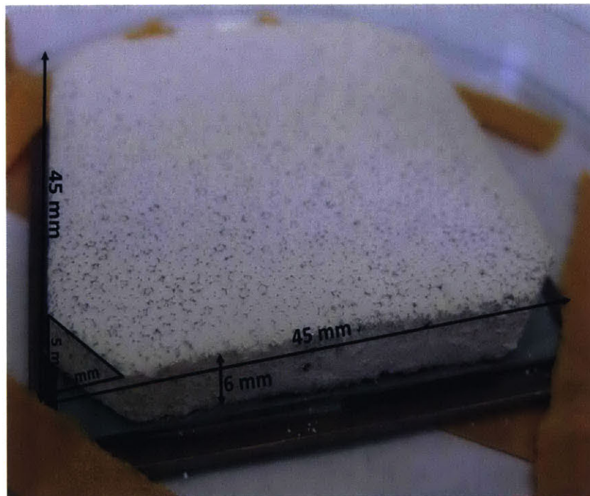
Figure 29: Picture of the sample of MgY zeolite in nickel foam that was installed into the adsorbent chamber of the Dual Chamber Prototype. Corners were cut off the sample to prevent interference with the fillets on the inside of the chamber.
