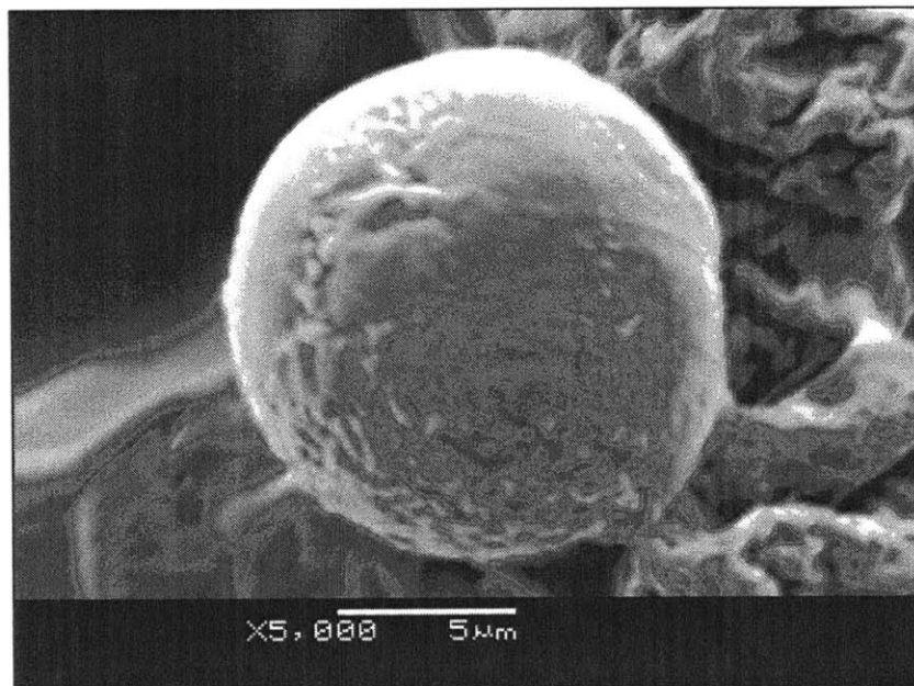
Figure 2.15: PMMA-POSS sprayed using an ultrasonic nozzle
