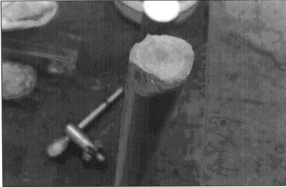
Figure 3.9: Fractured Mycalex rod
