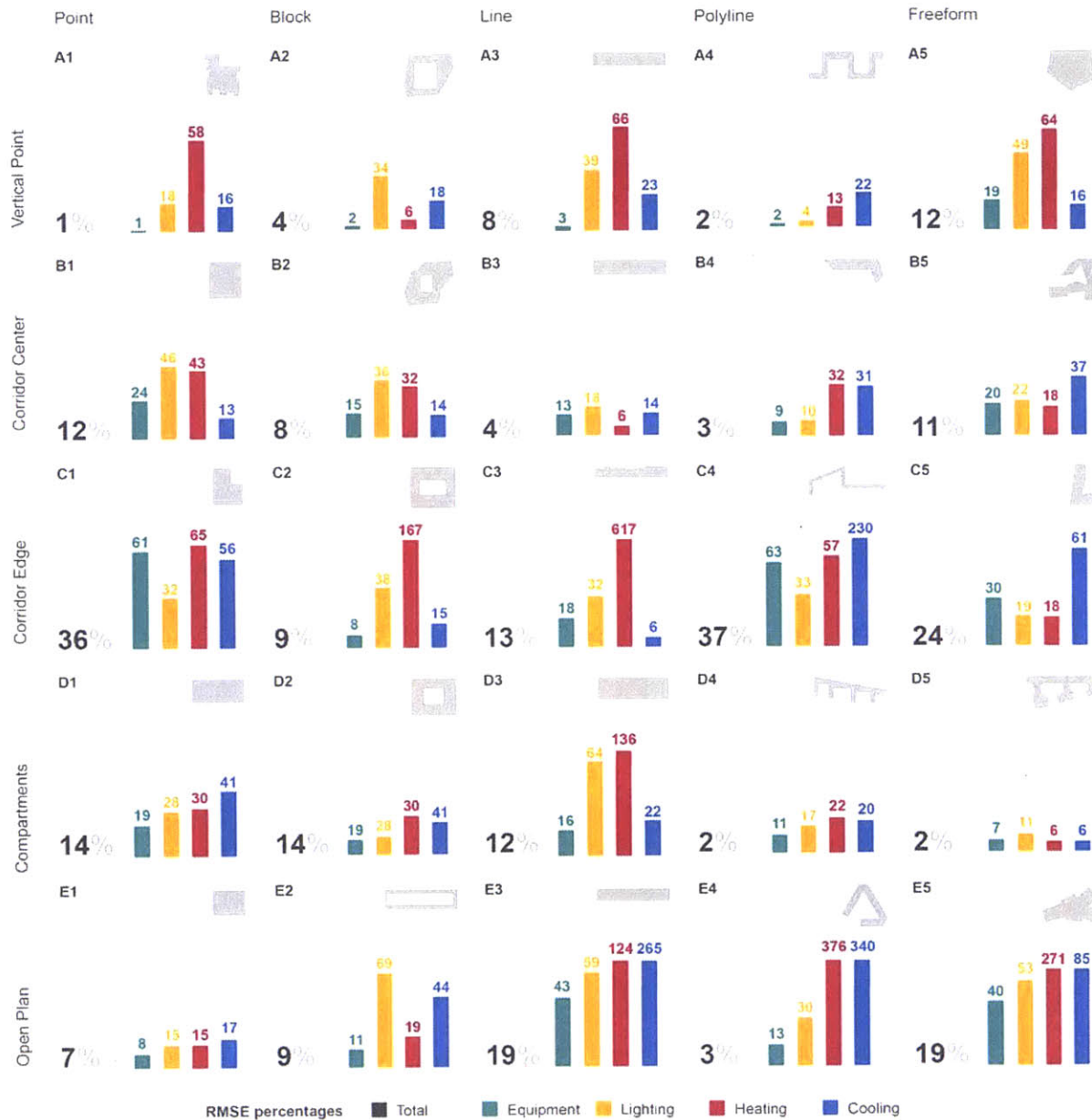
Figure 5-5 RMSE for EUI and sub-metrics plotted on the floor plan matrix.
