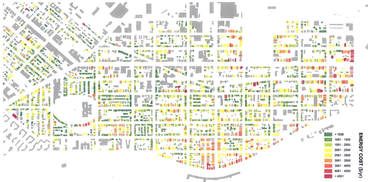
Figure 4-17: Energy simulation based energy cost predictions and potential urban “energy hogs” in magenta.
