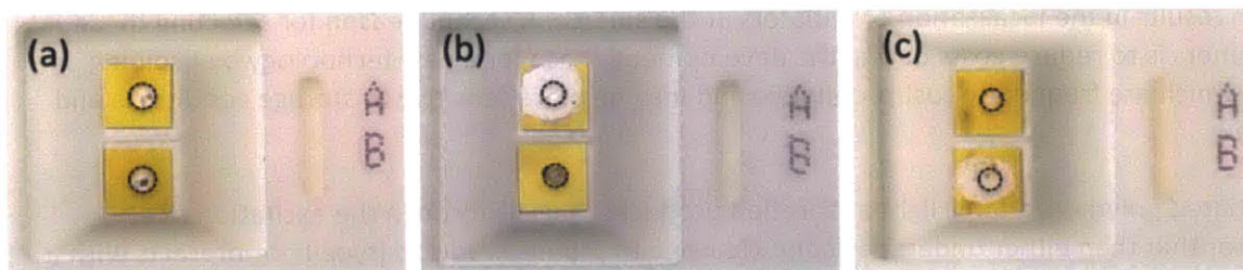
Figure 1-4. Subtyping influenza viruses with photopolymerization-based signal amplification. (a) No virus detected so polymer is only observed within the positive control spots. (b) Influenza A detected. (c) Influenza B detected. Reprinted with permission from Sikes et al., Lab on a Chip , 2009, 9, 633-656. Copyright © 2009, The Royal Society of Chemistry. 13
