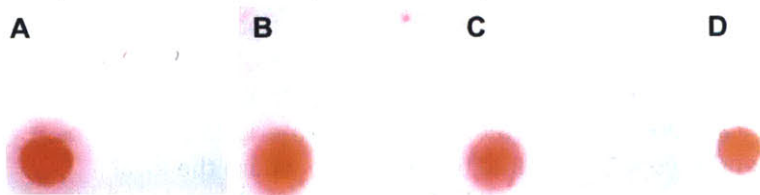
Figure 5-7. Negative and positive controls. (A) The test surface was prepared omitting the incubation with a biotinylated fibronectin clone. This demonstrates that nonspecific binding of streptavidin-eosin to EGFR does not result in a false positive. (B) The test surface was prepared with 1 \mu M unbiotinylated clone B in place of its biotinylated counterpart. (C) The test surface was prepared with 1 \mu M unbiotinylated clone E in place of its biotinylated counterpart. (D) The test surface was prepared with 1 \mu M unbiotinylated clone D in
