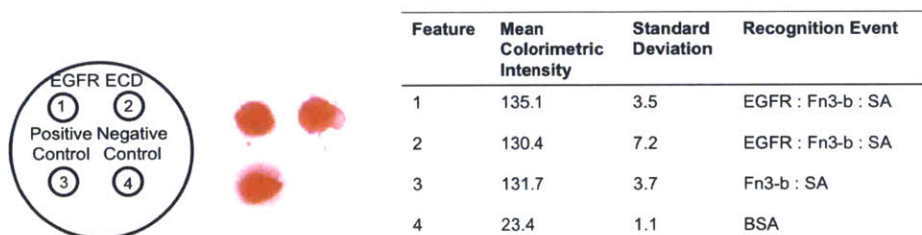
Figure 5-6. Colorimetric detection of clone D binding to surface immobilized EGFR. The concentration of clone D in solution was 1 \mu M. Features 1 and 2 are stained hydrogels generated in response to two subsequent binding events. First, biotinylated clone D binds to surface immobilized EGFR. This is followed by the binding of streptavidin-eosin. Feature 3 is a positive control for the polymerization reaction. In this case, streptavidin-eosin binds to biotinylated protein immobilized on the surface. Feature 4 is a negative control consisting of surface immobilized BSA. The mean and standard deviation values reported in the accompanying table derive from the quantification of the pixel intensities comprising each feature in the digital image and are based on areas incorporating the majority of each feature, but excluding edge effects.
