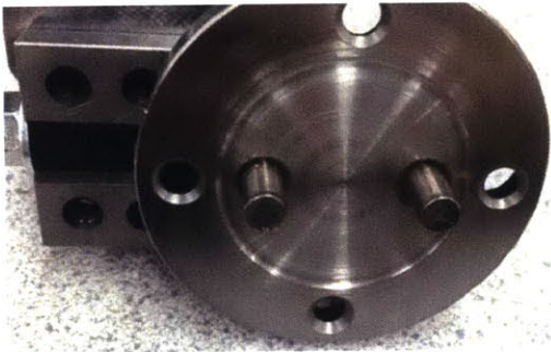
Figure 4-24. The rectangular base for OASIS system.
