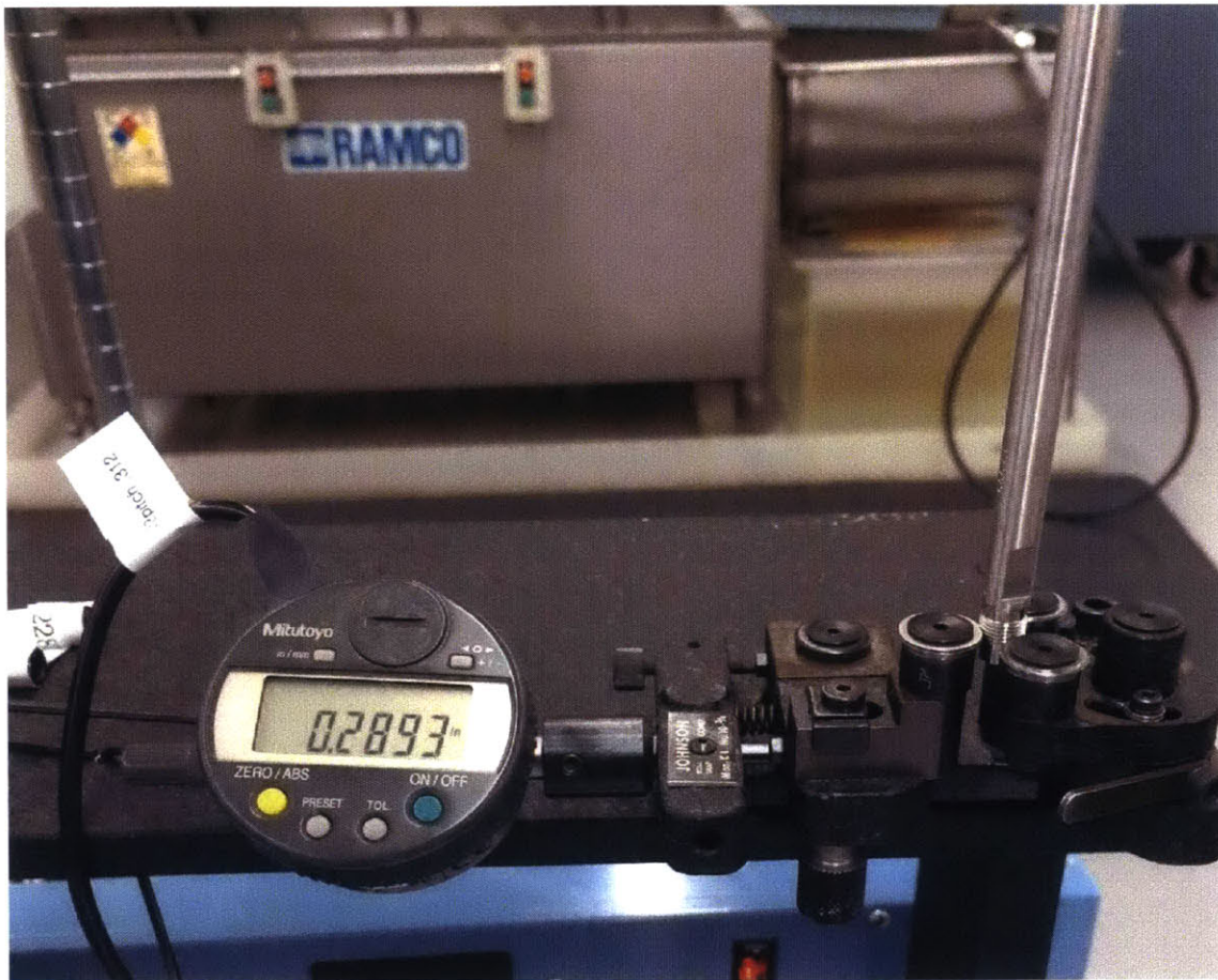
Figure 17: Johnson gage used to measure pitch diameter of thread.
