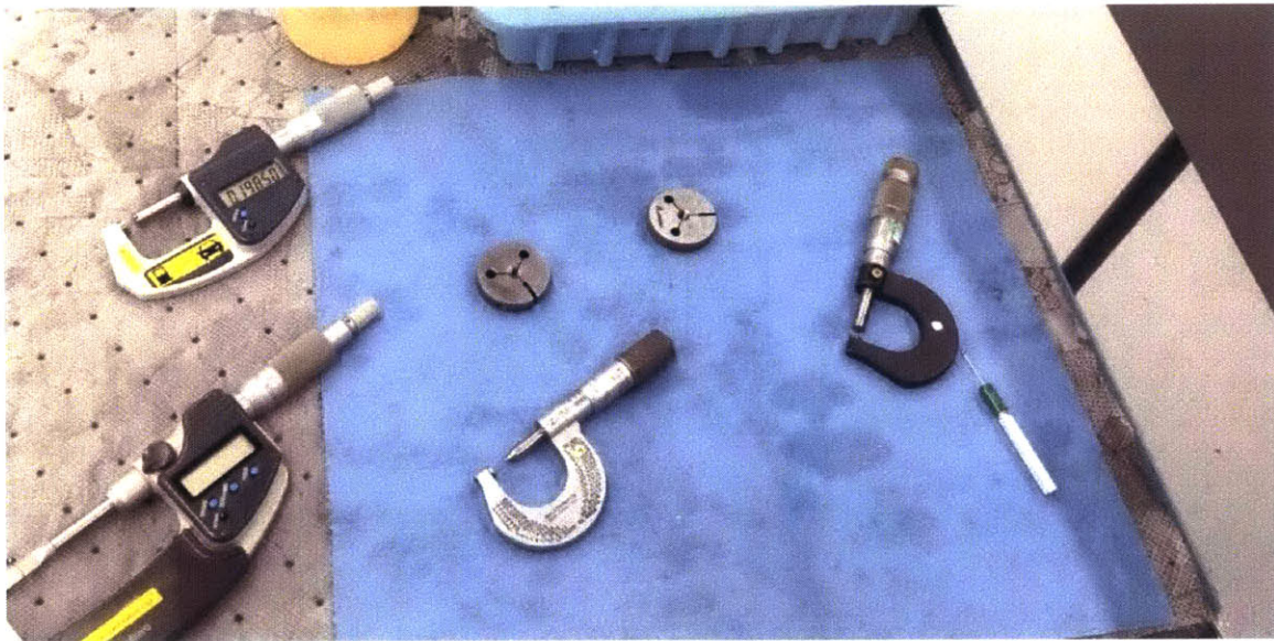
Figure 16: Quick check tools including blade micrometer, regular micrometer and go and no-go gages from left to right.
