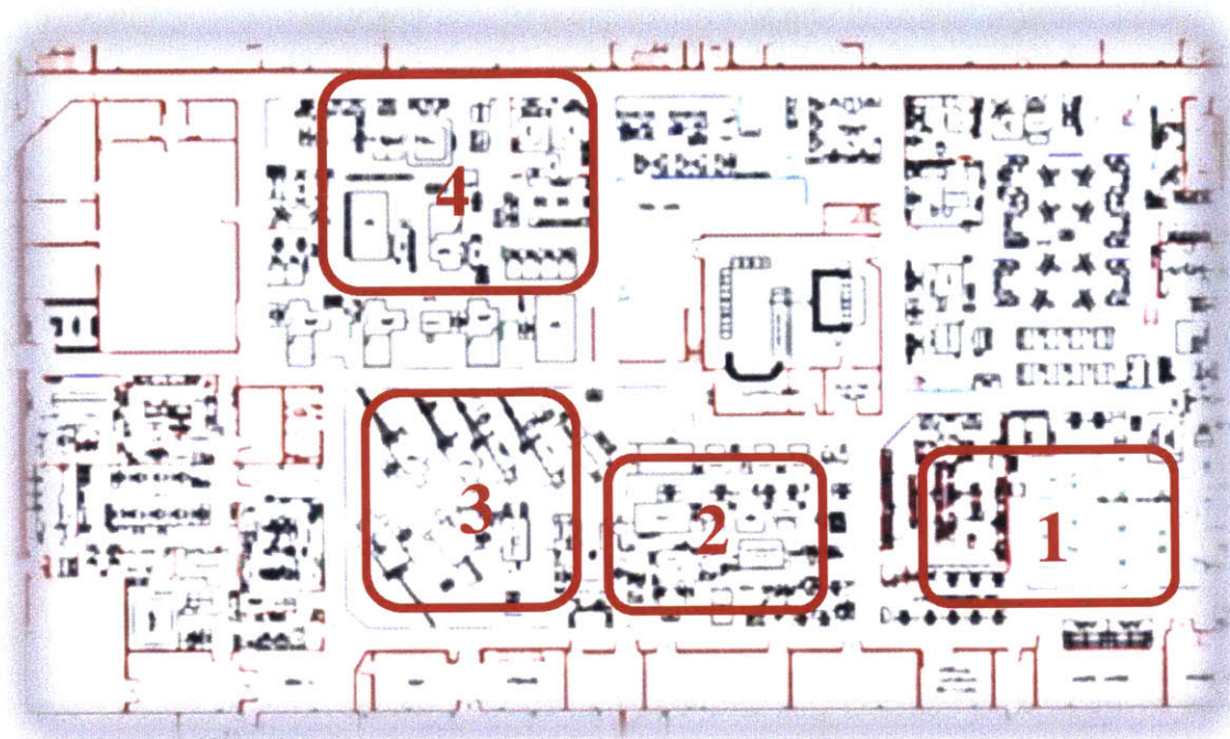
Figure 1: Waters global machining center layout. 1 = Column Area, 2 = Valve Area, 3 = NC Turning Area and 4 = NC Milling Area [3].
