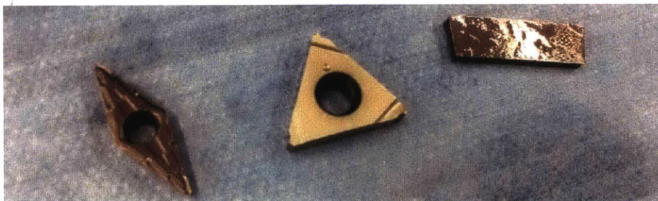
Figure 4: From left to right: turning insert, threading insert and cut off insert.
