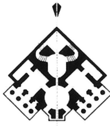
14-32. A floor plan of Montmorency Palace with bilateral symmetry, generated by substituting another procedure for Triangle in the code of Bilateral.
