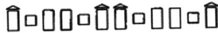
11-27. A complex fenestration rhythm generated by using the mod function and a case statement.
