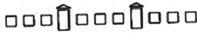
11-26. The use of modular arithmetic to vary every n th window in a row.
