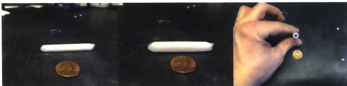
Figure S2. Hollow wax shell with cracks after removal from the glass rod (left). Hollow wax shell with the cracks repaired by dipping into molten wax (middle). Top view of a finished hollow wax shell (right).
