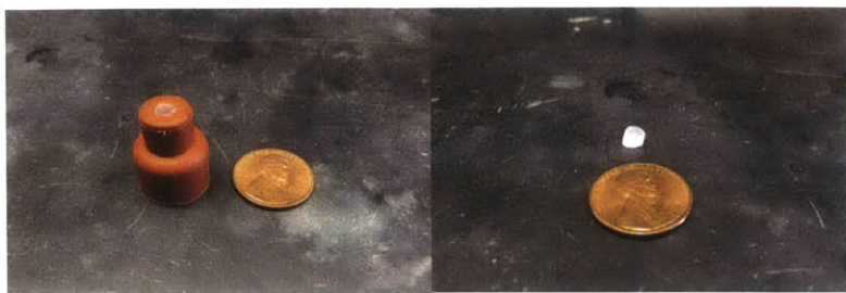
Figure S3. Filling the underside of a septum with a molten wax to create a wax cylinder (left). Wax cylinder once removed from the septa and trimmed to size (right).
