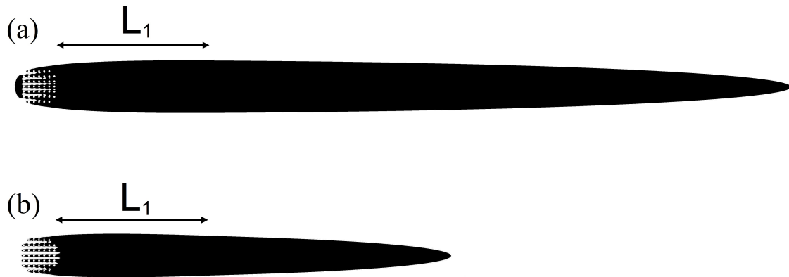
352 353 Fig. 9 The deposition area for a single patch ( A_1 ) is identified by the black color for two threshold velocities: (a) u/U_0 354 < 0.7 , A_1 = 22.7D^2 ; (b) u/U_0 < 0.5 , A_1 = 9.9D^2 .
