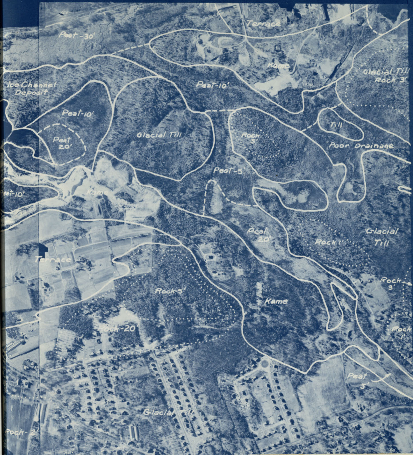
FIGURE II AIR PHOTO MOSAIC SOIL MAP OVERLAY RELOCATION OF ROUTE 28 0 400 800 FLOWN DEC. 3 1952 BY JACK AMMAN PHOTOGRAMMETRIC ENGRS PART OF CONTRACT 5244 FOR MASS. DPW.
