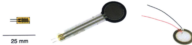
Figure 2-3: Electrical paradigms for measuring force including a representative strain gauge ( Left ) [32], FSR ( Center ) [31], and piezoelectric transducer ( Right ) [33].
