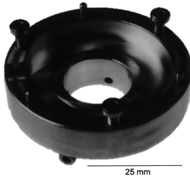
Figure 3-2: This image shows the prototype adapter. This part connected the flexure system to the actuator housing.
