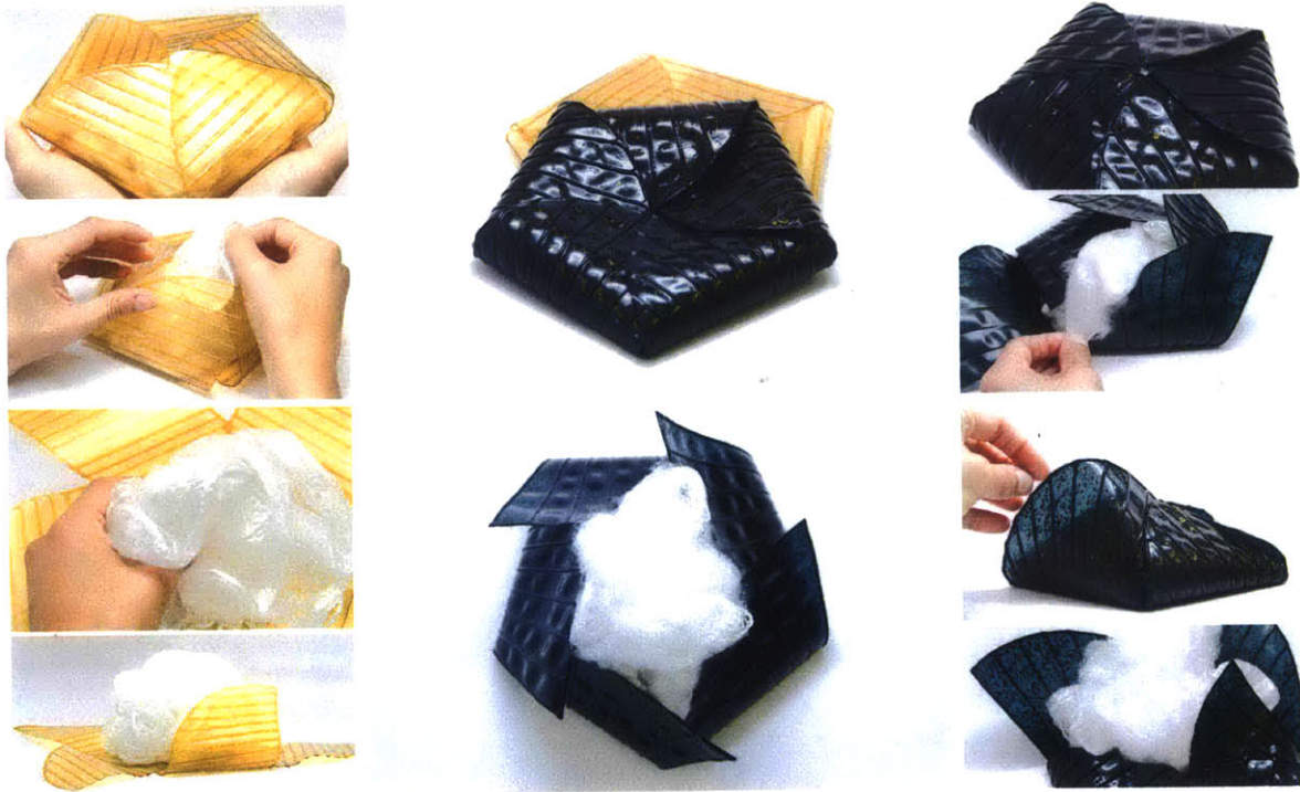
Figure 3-20: Bioplastic-based fully recyclable packaging products composed of plasticized CHI 10% concentration and plasticized CHI 10% concentration with black food coloring additive.
