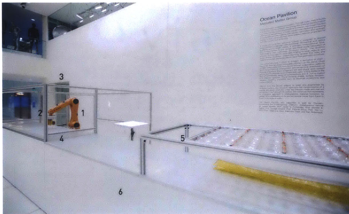
Figure 3-8: Perspective view of the manufacturing platform installed at the MIT Media Lab composed of (1) a positioning robotic arm (Kuka KR AGILUS robotic arm, model KR 10 R1100); (2) a customized multi-barrel extrusion head for water-based materials; (3) a security envelop for operation of the robotic assembly; (4) a 1m-wide and 5m-long deposition bed; (5) a computer-controlled evaporation system composed of 100 fans; and (6) a 9m-long workspace and storage cabinet. Figure from Mogas-Soldevila et al. [2015a].
