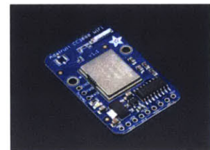
Adafruit breakout board for the CC3000 wifi module from TI.
