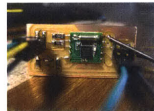
Milled circuit board for testing the FM radio module.
