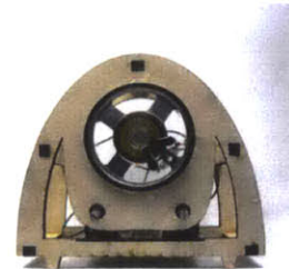
Fab FM plywood frame w/ electronics.
