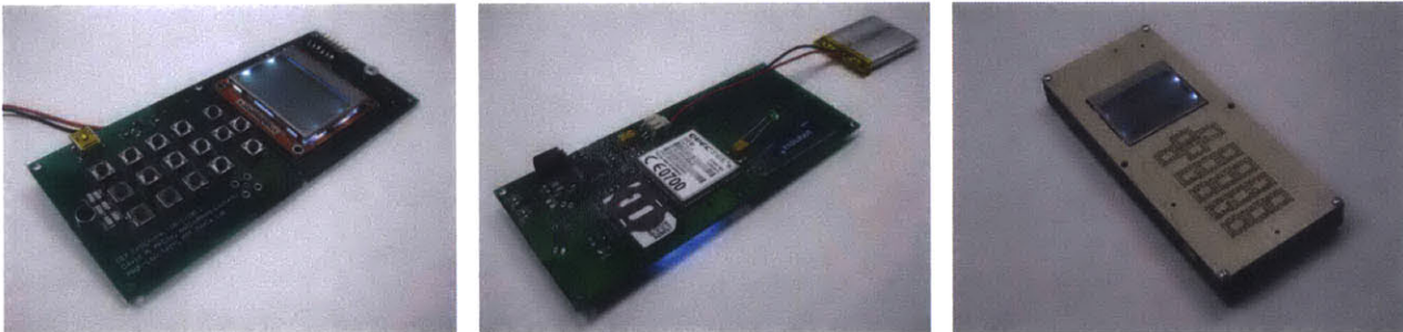
The first DIY cellphone that I used in my daily life: circuit board (left and middle) and laser-cut enclosure (right).
