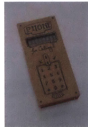
Phones made by friends: 3D-printed enclosure by Amit Zoran (top); hand-cut and illustrated cardboard enclosure by Jeffrey Warren (bottom).
